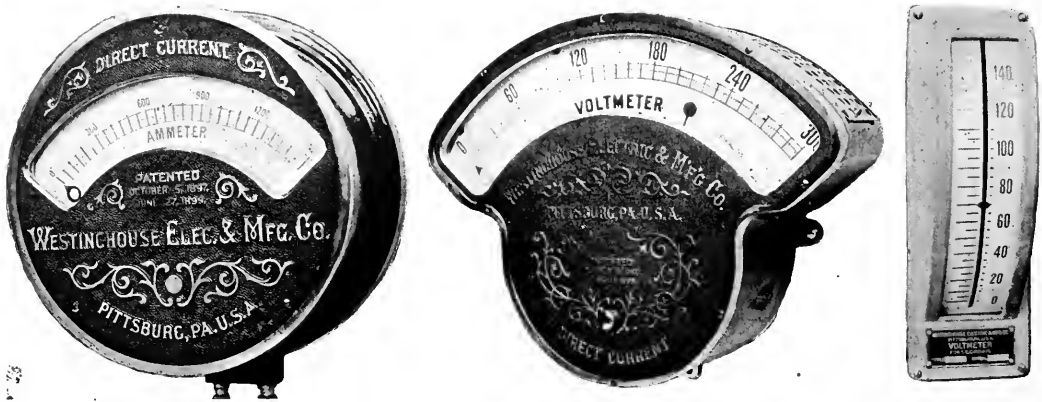
FIGS. 1, 2 AND 3.—DIRECT-CURRENT SWITCHBOARD INSTRUMENTS.
